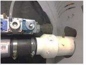
3. Remove the venturi/gas valve assembly from the blower by removing the 3 screws using a T30 Torx driver. Save the screws for reinstallation.
