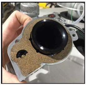
6. Install the orifice onto the gas valve.
