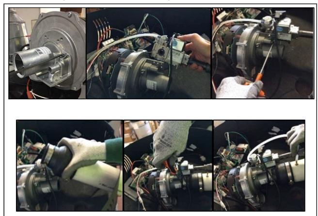
8. Connect gas and electrical supply to the water heater and check for gas leaks. Adjust the CO<sub>2</sub> percentage to the appropriate model data given in table 1 when water temperature is 55°C. Turn venturi screw counterclockwise to increase CO<sub>2</sub> percentage, and clockwise to
