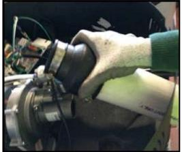
3. Loosen the 3 screws that attach the gas valve to the venturi with 5/32" (4 mm) Allen drive. Remove the gas valve from the venturi. Save the screws for reinstallation.
