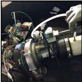
2. Loosen the air intake clamp. Remove the air intake from the venturi.
