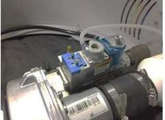
2. Remove the gas valve reference tube from the intake.
