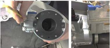
5. Install the inner O-Ring and the orifice included with the kit.
