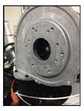
5. Install the cork gasket onto the new venturi included in the kit.
