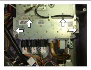
(3) Pull up and remove the manifold.
