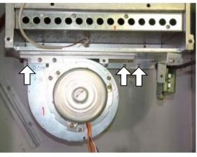
(2) Remove the 2 case top plate locking screws.
