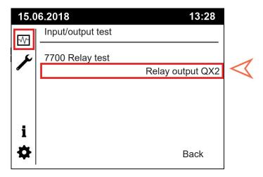
Using the control knob select field "7700 Relay test" and press control knob. Rotate the control knob to select output to test. Press the control knob to activate the desired relay (see example above).
