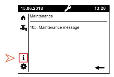
In this example '105: Maintenance message' is used to notify the user, the heater has been in operation for more than 12 months and requires a service inspection. When servicing has been completed, the service counter should be reset using parameter 7045, in the Service / special operation menu (see section 4.4 for details)
