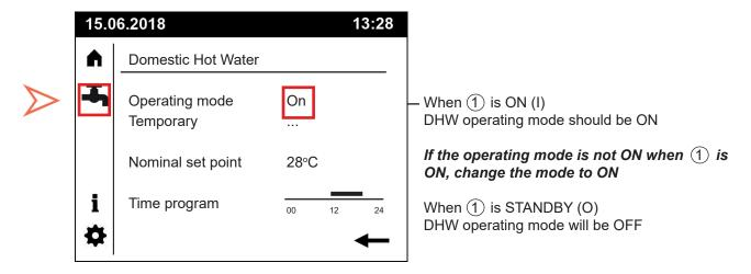
With the DHW tab selected, rotate (3) to highlight the time program field,
