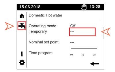
Rotate the control knob to change the "Temporary" field from "..." to "Recharging" and press the control knob to select the value
