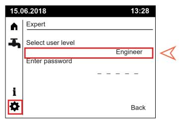
Select "Engineer" using the control knob and press the control knob to select it. Press control knob to continue into commissioning mode.
