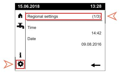
Turn the control knob to highlight regional settings and push the control knob to select. Turn the control knob to select one of the 3 setting pages. Push the control knob once the desired page is selected and rotate the control knob to select the required field.
