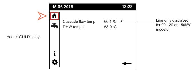
The start page for the heater GUI unit displays the most important information on the water heater and system operation mode. There are no settings that can be applied whilst in this screen.
