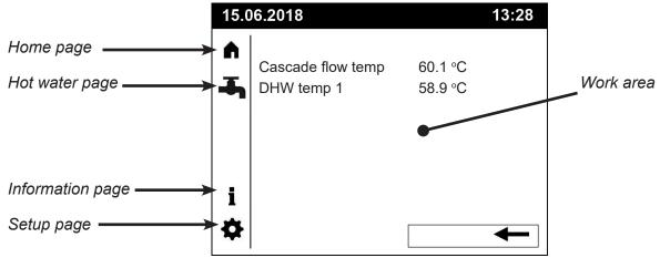
The water heater is operated by rotating the control knob to move the selector over the screen then pushing the control knob to select the item. When selected the item will be displayed as inverse and can then be changed by rotating the control knob and the change is confirmed by pushing the control knob.
