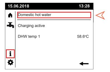
To view further pages select the " **1**" page and press the control knob. The field at the top of the screen can now be selected with the control knob and rotated and selected again for the info page required. See example: -
