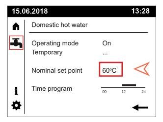
Once the field is selected rotate the control knob to change the Domestic Hot Water set point. Confirm the selection by pressing the control knob within 3 seconds.
