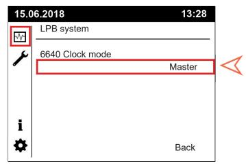
If the optional web server is fitted this setting will need to change to "Slave with local setting", as the web server will act as the time clock master and will provide all of connected heaters with a common time taken from the internet. No adjustment for summer and winter times will be necessary if the web server is installed, as time adjustments will be carried out automatically.
