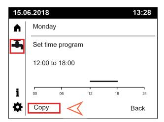
After setting up the times of the day required to be copied, rotate (3) and select copy in order to move to the "copy to screen".
