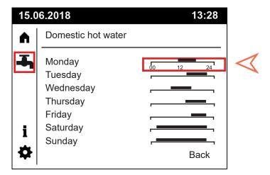
Turn and push the control knob to set the start and end times of the program. Scroll to the beginning (00 hours) to insert another time band (up to a total of 3 time bands per day can be set).
