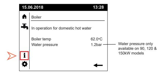
On a 90, 120 or 150kW model the "Cascade" screen will display the combined flow temperature of both operating heat engines and this represents the temperature of the water being charged into the tank. On a 30kW or 60kW model "Boiler temp" represents the temperature of the water being charged into the tank.
