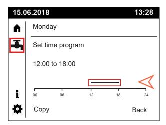
To delete a time band use the control knob to move the start and end times of the band to be the same then press the control knob.
