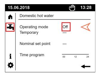
When operation switch is set to position I (ON), DHW operating mode should be ON (see example below)
