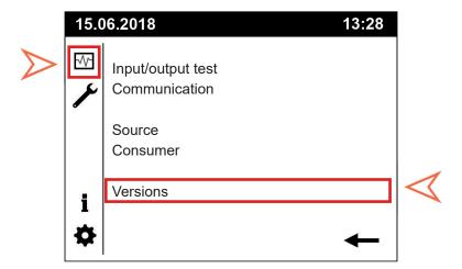
Details are shown for the software and text versions being used by the GUI, this may be useful to establish the level of updates applied to the heater.
