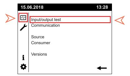
Highlight "Input/output test" using the control knob and select the function by pressing the control knob
