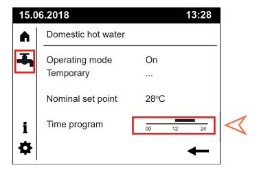
Press ③ to enter the time clock setting page. Once the field is selected rotate ③ to reach the time programming screen.
