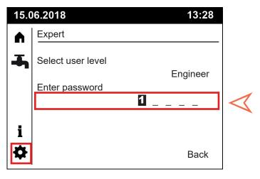
Enter password '10001' by rotating the control knob, and then pressing the control knob to input each number.
