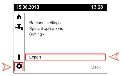
In the work area, use the control knob to select "Expert" field and press the control knob to select
