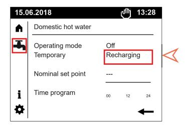
The heater operation in now active and will recharge the DHW tank water to the nominal set point previously programmed
