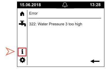
In this example the heater has gone into lockout mode, because the primary system pressure has exceeded 9.0 bar. The resolution would be to rectify the overpressure condition and reset the error to restart heater operation again (see below)
