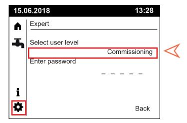
Select "Commissioning" using the control knob and press the control knob to select it. Press control knob to continue into commissioning mode.
