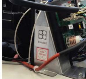
3. Peel off one side of a sticky fixer and stick it over the terminal block symbol on the "Enable" label (see photo below)
